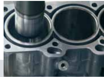
PCBN insert Cylinder boring (rough & finish)
