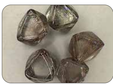
A: OCTAHEDRON Point angle 90 degree / Applications : SDD, Natural diamond-MDD
